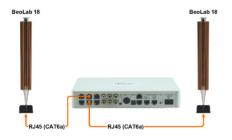
Newer B&O speakers can be connected with RJ45 patch cables (CAT 7). If the speaker has two Powerlink RJ45 sockets, you can also loop the cables through (daisy chain).
