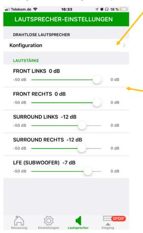
This button takes you to a page for wireless connection of speakers with WISA module (e.g. newer B&O loudspeakers such as BeoLab 18). Note: This function is only available if the almando Multiplay Surround Switch has an integrated WISA module (option with additional costs).
