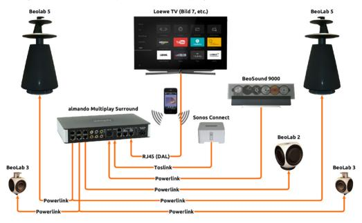
Powerlink signals from connected B&O devices are simply looped through. All other audio signals - whether digital or analog - are converted to a 100% standard B&O Powerlink signal including the trigger voltage required for the B&O loudspeakers (as well as the B&O data signal for BeoLab 5, BeoLab 4500 and BeoLab Penta if required).
