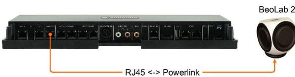
Subwoofers like a BeoLab 2 are connected to the RJ45 subwoofer socket.
