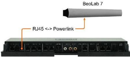
The RJ45 center socket is specifically designed for connecting center speakers only. The center tone is output on both Powerlink audio signals from this socket. This makes it possible to connect not just mono but also stereo speakers (as shown here with a BeoLab 7).
