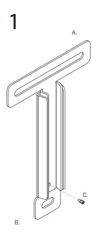
The length of A. and B. combined can be adjusted to suit the requirements of the TV and the soundbar.
