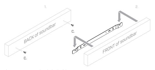
The C. screws are used on the back of the soundbar and afterwards fitted into the wall bracket.
