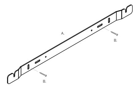
The B. screws are used to install the backet on the wall.
