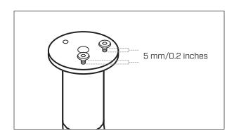
Don not screw all the way to the bottom. Leave a small gap of approximately 5 mm/0.2 inches.
