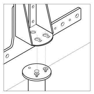
Gently align TV and top of BS19 to the bottom part. Then lower the TV and top of BS19 so the two screws passed through the 'keyholes'.
