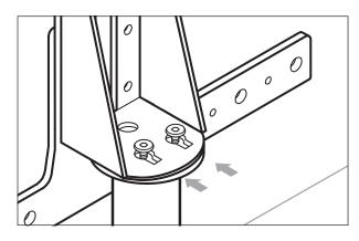
Gently push the TV and top of BS19 so the two screws are positioned in the narrow end of the 'keyholes'.
