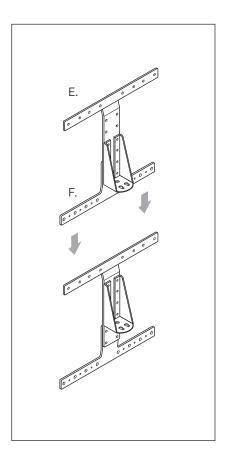
You can change the initial height of the TV on BS19 by adjusting the position of D. and E. on to F. This option requires additional screws which need purchase. J1./J2 J1./J2 J1./J2 J1./J2 E. Adjust the position of F. and E. according to the specs of the TV.
