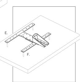
You also change the initial height of the TV on BS19 by swopping the position of D. and E. on to F.
