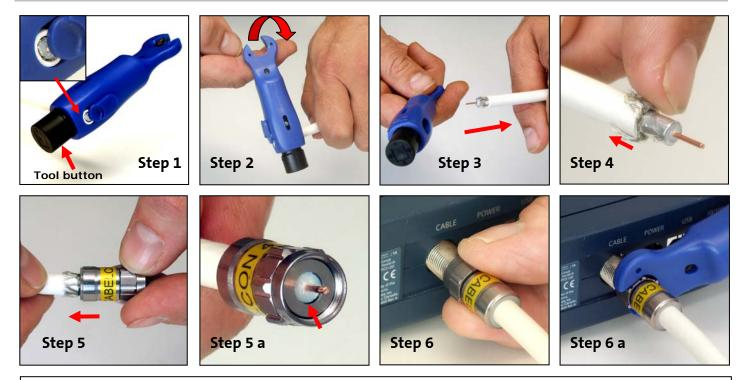
STEP 1: Press and hold the black button and insert cable until the mechanical stop as shown. Release the button.
