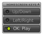
To configure the **OK** button, select the bottom entry and use **LEFT** and **RIGHT** arrow keys to switch between *Menu* and *Play*. The former allows the **OK** button to bring up the menu (default), the latter changes the **OK** button to act as a Play / Pause button in the USB mode.
