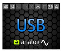
The default home screen view consists of three components. The currently active input is displayed at the center.
