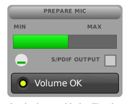
➤ The microphone check screen appears. At this point, plug in the provided calibration microphone to the microphone jack and position it at the primary listening spot. The microphone should be positioned at ear height, with no reflective surfaces near the tip and fixed in place.
