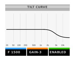
✓ Enabled: Enables or disables the applied tilt curve.
