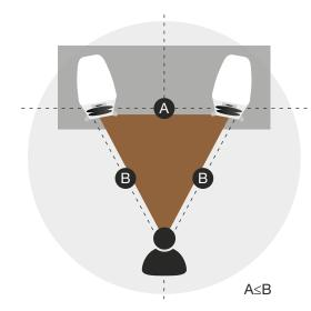
Fig. 3 - Positioning the loudspeakers.
