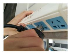
Plug in the screen power, press the "up" button of the RF remote within 3 second until the LED light flash.
