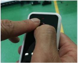
Confirm whether the weight bar is moving(down> up), if the weight bar is down a little, then up, that is to say, the RF remote is synchronized with screen.
