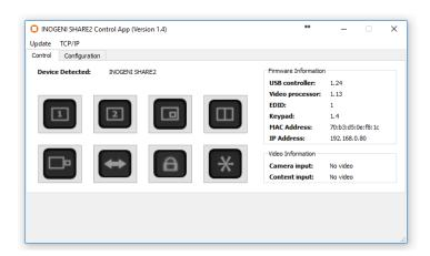
The device has its own application in order to control the Mixer configuration using the USB Human Input Device (HID) or the LAN interfaces.
