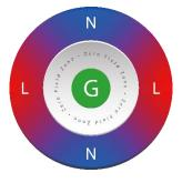
SilentPower's Ground Zero technology is a unique feature in their power cables. Here, the ground wire is surround by live and neutral wires in a geometrically balanced pair. The shotgun configuration of the ground conductor prevents the ground wire from being affected by magnetic fields, and the balanced design maintains constant impedance regardless of whether the cable is angled or bent – ensuring pure mains electricity feeds into your audio or AV system.
