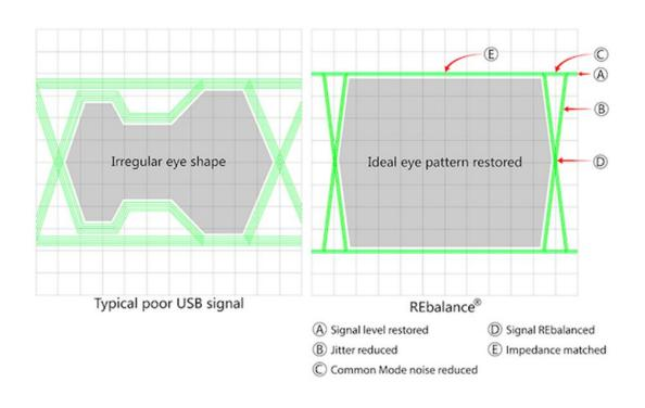
The REBalance technology inside the iSilencer Max rebalances the USB signal to address DC offset and jitter, leading to distortion, and in turn, data packet errors.
