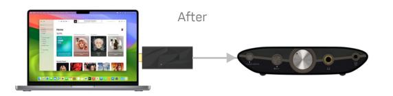
A computer power supply's USB bus is often sourced from an inadequately filtered switch-mode power supply, that injects noise into connected equipment – leading to data errors, loss, and jitter.
