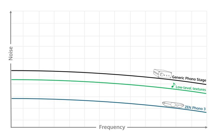
The noise floor of a typical phono stage is noticeable. This is because it sits **above** the level of the low-level textures and detail of the music.
