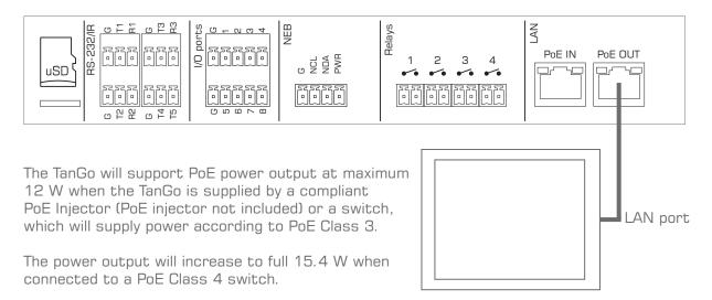
Be aware that the cable length and cable quality will impact how much power can be drawn by the connected device at the PoE OUT terminal. This is due to the fact that the TanGo will monitor the power loss in the cables and shut down the output if this loss is too high.
