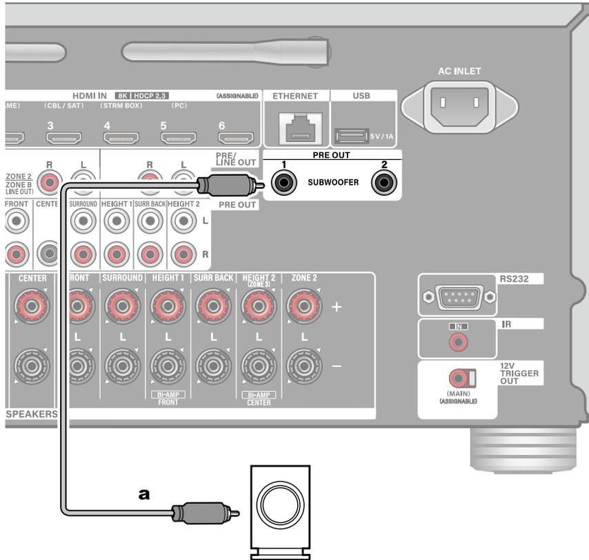
Connect a powered subwoofer with this unit using a subwoofer cable. Up to two powered subwoofers can be connected.
