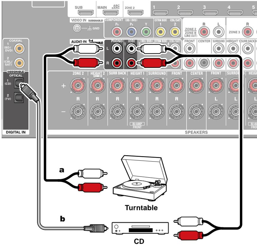
This is a connection example of an audio component. Connect a CD player using an analog audio cable. You can also connect a turntable that has an MM-type cartridge to the PHONO jack.
