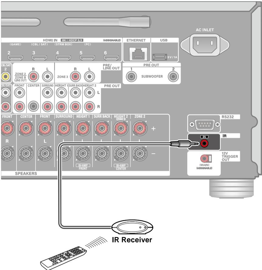
When connecting a remote control receiver unit consisting of an IR Receiver, etc. to this unit, operation using the remote controller is possible even if the remote control signal is difficult to reach (due to installation in the cabinet, etc.). You can also operate the unit using the remote controller from a separate room such as ZONE 2. For installing a remote control receiver unit, contact the specialized stores.
