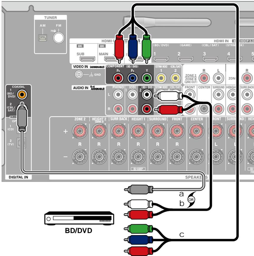
a Digital coaxial cable, b Analog audio cable, c Component video cable
