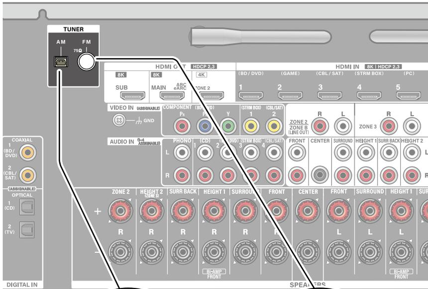
Connect the antenna to this unit, and set up the antenna at the best position for listening while receiving radio signals. Attach the indoor FM antenna to the wall using push pins or adhesive tape.
