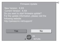
Select "Yes" to start downloading the firmware. When the firmware update starts after the downloading is finished, a black screen is displayed.
