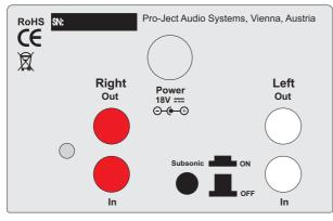
Make all connections whilst the phono amplifier is disconnected from the power supply.
