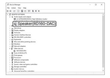
• 3-3-5. When you set the sound device to RD160-DAC in the system tray area of your PC, you are ready to use the device connected to the USB IN port.
