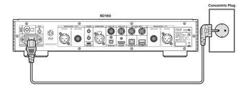
⚠ Caution: When disconnecting the power cord, always disconnect the power outlet first with the power switch off.
