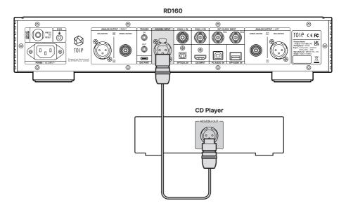
• You can connect the digital output port of an external device to the 12S input port of this product as shown in the figure below.
