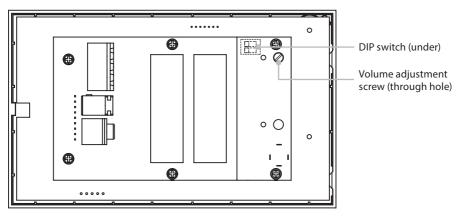
Rear panel controls for installer adjustments
