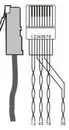
**Notice:** Cable connectors MUST be metal one, the shielded layer of cable MUST be connected to the connector's metal shell, to make a better transmission.
