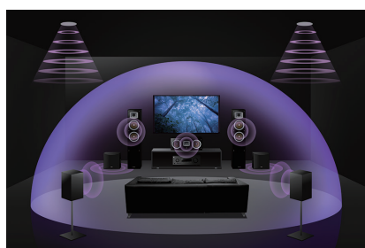
5.2.2-channel with in-ceiling speakers
