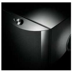
The cabinet employs a massive 19kg (41.9 lbs) high strength, heavy bass reflex enclosure constructed of thick 36mm (1-3/8") MDF (medium-density fiberboard) on the baffle sides and 25mm (1") MDF on the other sides with traditional three-way mitered-joint construction. It has a strong resonance-resisting structure with cast-iron legs and a front-firing design with the woofer unit attached to the front of the enclosure. It delivers direct, razor-sharp sound that's ideal for high-end audio systems.
