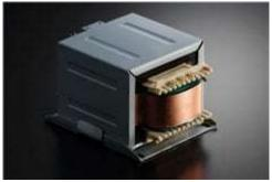
The huge power supply for the built-in power amplifier has a massive 10.2kg (22.5 lbs) high capacity power transformer and two large 160V 4,700µF block electrolytic capacitors, making it capable of sustaining the 1kW power output. Yamaha used a conventional pure analog power supply to achieve superior response and musicality in the very low bass range.
