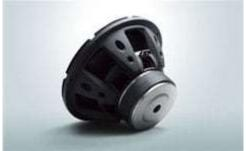
To achieve long-stroke drive with its superior linearity, the NS-SW1000 uses a 30cm (12")woofer unit with a strong, flexible drive system employing double layer large diameter ferrite magnets and a double damper with an air vent. The frame is high strength aluminium diecast to suppress unwanted resonance even at high volumes, making it possible to reproduce delicate tonal nuances.
