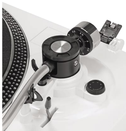
The cue lever is too close to the arm rest clip.
