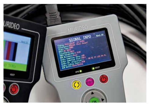
Murideo test equipment give very specific classification information for each cable, allowing us to determine if a cable will meet required standard. It will show if the cable is able to transmit desired standard and if 18Gbps is needed or if the lower speed class is sufficient for desired media transmission.
